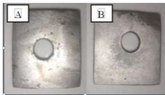
Figure 8. Surface morphology of steel after 6 days of immersion with 20% inhibitor (A) in seawater (B) and 25% CH 3 COOH
